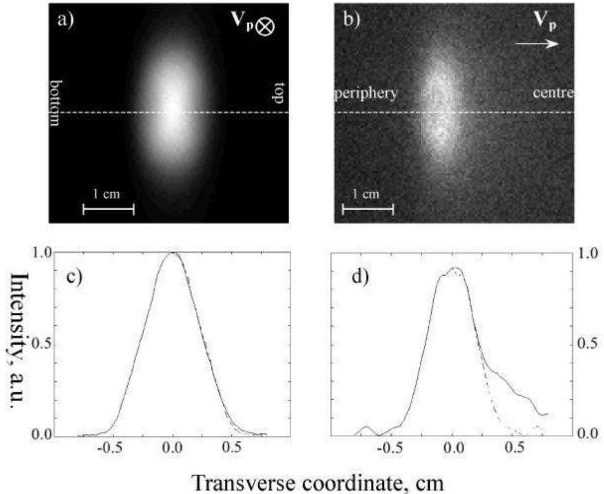
Fig. 1. a), b) The snapshots of the carbon pellet cloud in #49982. c), d) The corresponding intensity profiles in the central cross-section.
