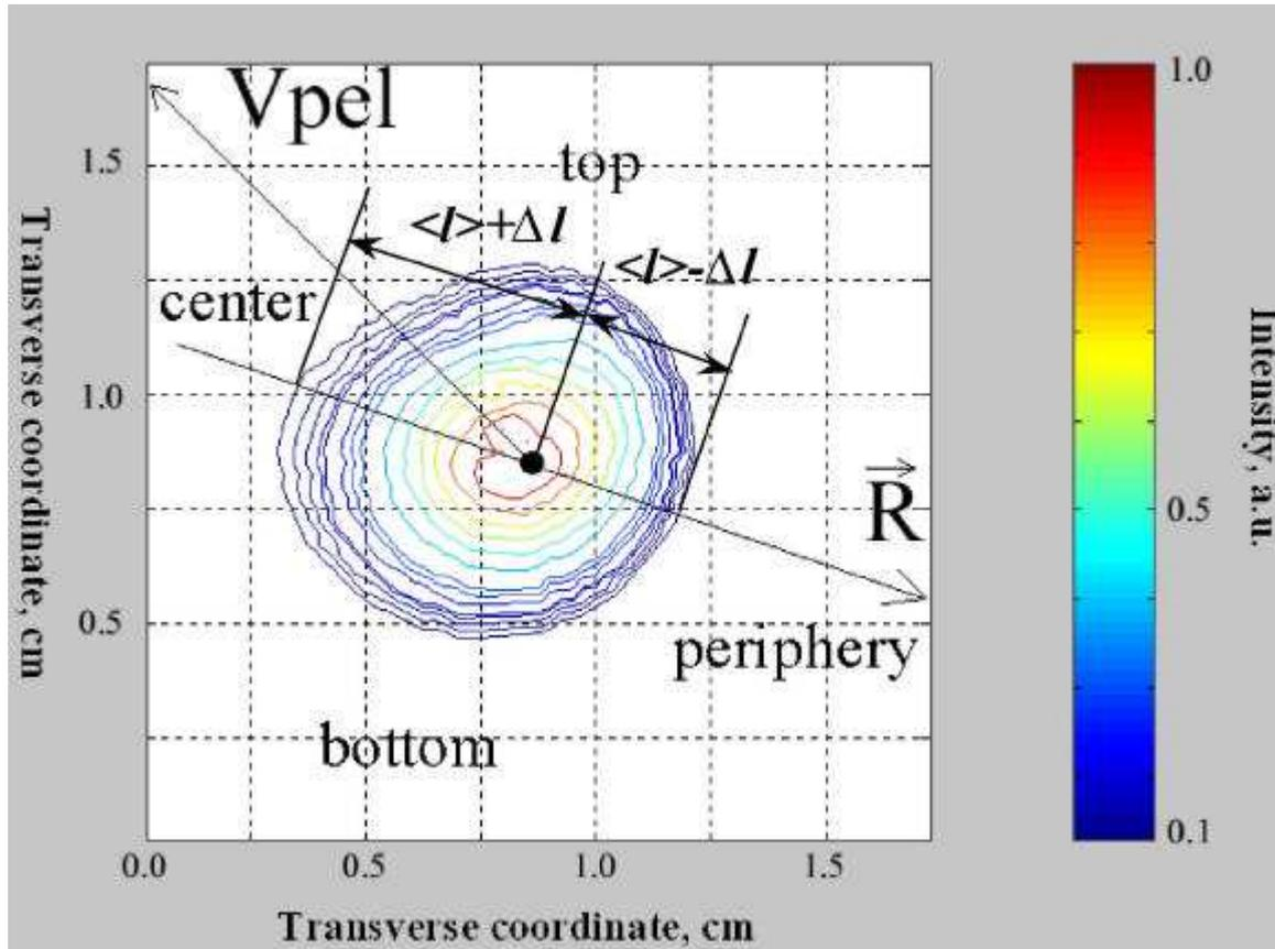
Fig. 2. An example of the restored intensity distribution for shot #49982 in the cross-section passing through the cloud center.
