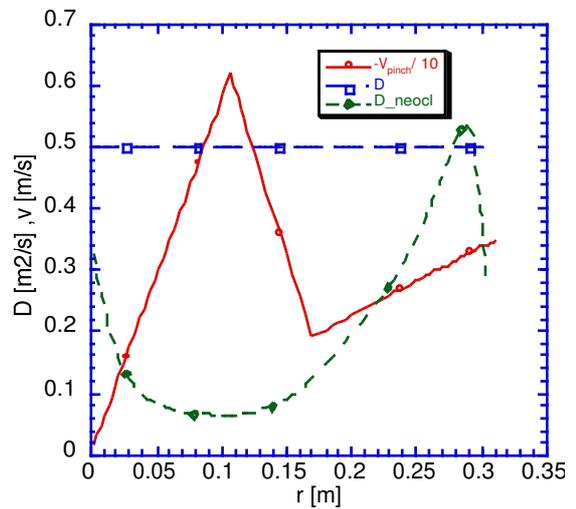
Fig.7 Transport parameters used to simulate ITB discharges and the neoclassical diffusion coefficient.
