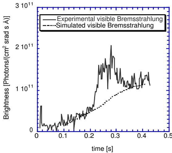
Fig5 Experimental and simulated Bremsstrahlung brightness in the visible range versus time (#20859)
