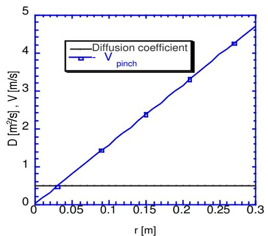
Fig.2 Profiles of diffusion coefficient and pinch velocity (inward) used to well simulate Ne seeded and unseeded discharges
