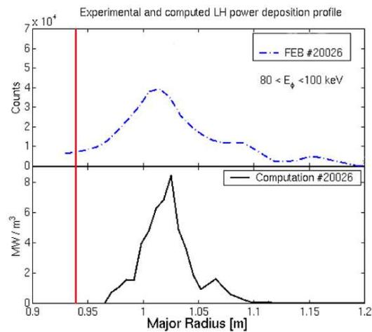
Fig. 7. Experimental deposition profile from FEB camera compared to the theoretical prediction from a Bonoli type code. The vertical line is the plasma centre.
