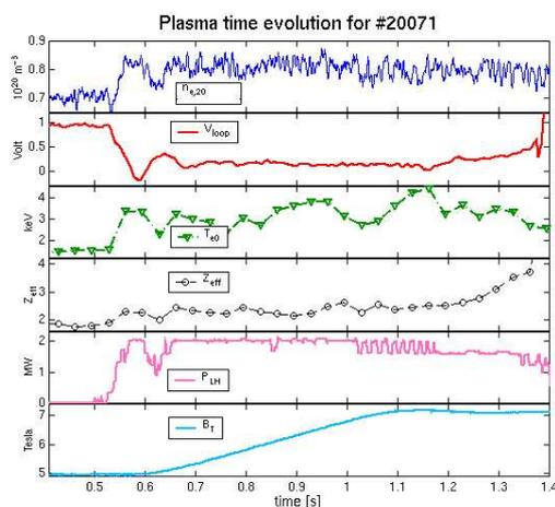
Fig. 1. Discharge #20071,  $I_p = 0.36 \text{ MA}$ , swinging  $B_t$ . Temporal evolution of density, loop voltage, electron temperature,  $Z_{eff}$ , LH power and toroidal field. .
