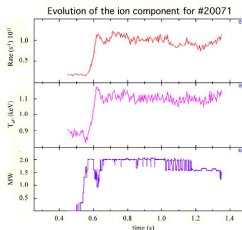
Fig. 2. Discharge #20071,  $I_p = 0.36 \text{ MA}$ , swinging  $B_t$ . Temporal evolution of ion component: neutron rate, temperature, LH power
