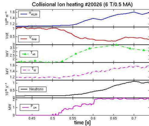
Fig. 3. Discharge #20021,  $I_p = 0.50$  MA,  $B_t = 6$ T. Temporal evolution of density, loop voltage, electron temperature, ion temperature, neutron rate and LH power.
