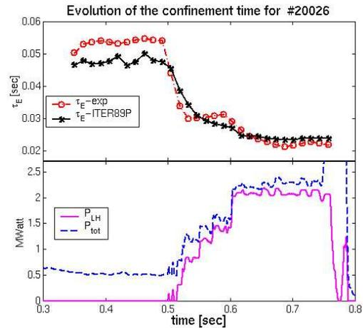
Fig. 6. Comparison between the experimental confinement time and the ITER89P scaling, LH and total power in the second frame
