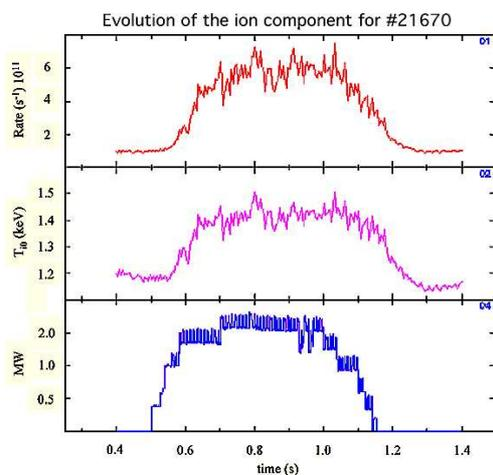
Fig. 5. Discharge #21670,  $I_p = 0.36$ MA,  $B_t = 7.2$ T. Temporal evolution of ion component: neutron rate, temperature, LH power
