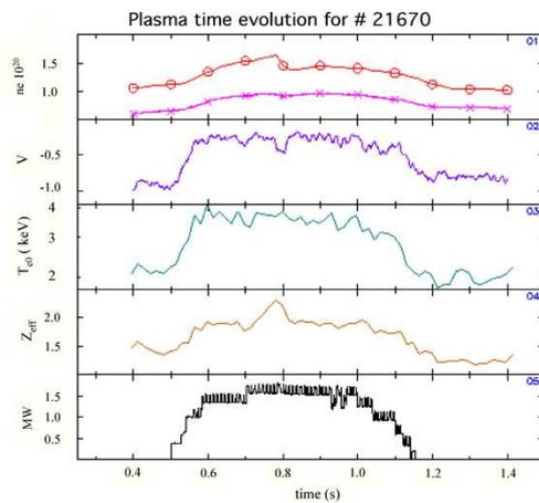
Fig. 4. Discharge #21670,  $I_p = 0.50$  MA,  $B_t = 7.2$ T. Temporal evolution of peak and average density, loop voltage, electron temperature,  $Z_{eff}$ , and LH power.
