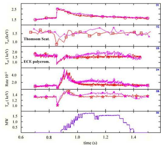
Fig. 8. Discharge #21802 (without LH), 21831 (with LH),  $I_p = 1.1$ MA,  $B_t = 7.2$ T. Temporal evolution of density, electron temperature from Thomson scattering and ECE polycromator, neutron rate, ion temperature and LH power
