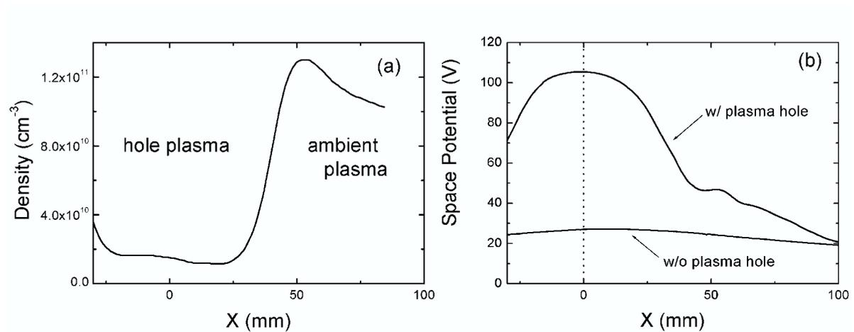
**Figure 1** (a) Density profile of the plasma hole. (b) Potential profile of the plasma hole. Potential profile without plasma hole is also plotted.
