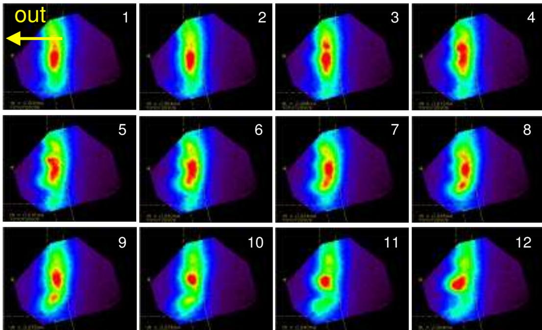
Fig. 2 – Edge turbulence images from Alcator C-Mod at 250,000 frames/sec showing a region  $\approx 6$  cm x 6 cm near the outer midplane with the outer wall toward the left.
