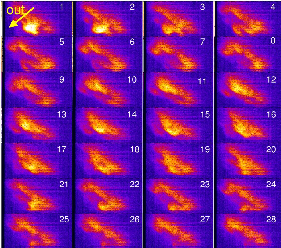
Fig. 1: Edge turbulence images from NSTX at 100,000 frames/sec showing a region  $\approx 30$  cm x 15 cm near the outer midplane with the outer wall toward the lower left corner.
