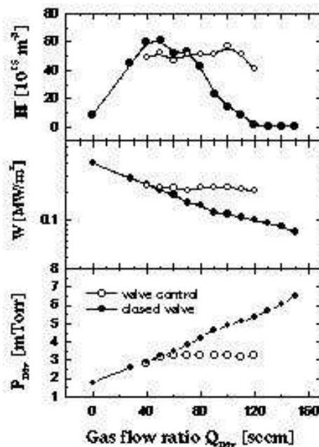
Fig.3 Typical characteristics of  $P_{Div}$ ,  $W$  and  $H$  on the gas flow ratio  $Q_{Div}$ .
