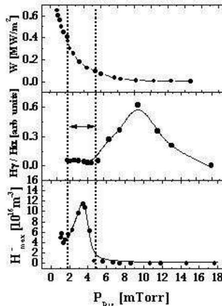
Fig.2 The dependence of  $W$ ,  $H_\gamma / H_\alpha$  and  $H_{max}^-$  on hydrogen gas pressure  $P_{Div}$ .
