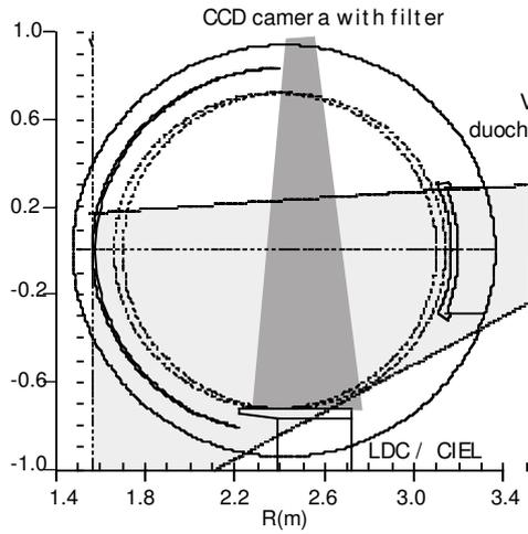
Figure 1. Schematic plan of viewing geometry for wide area CCD and fibre spectroscopy (vertical) and poloidal profiles from the VUV duochromator.
