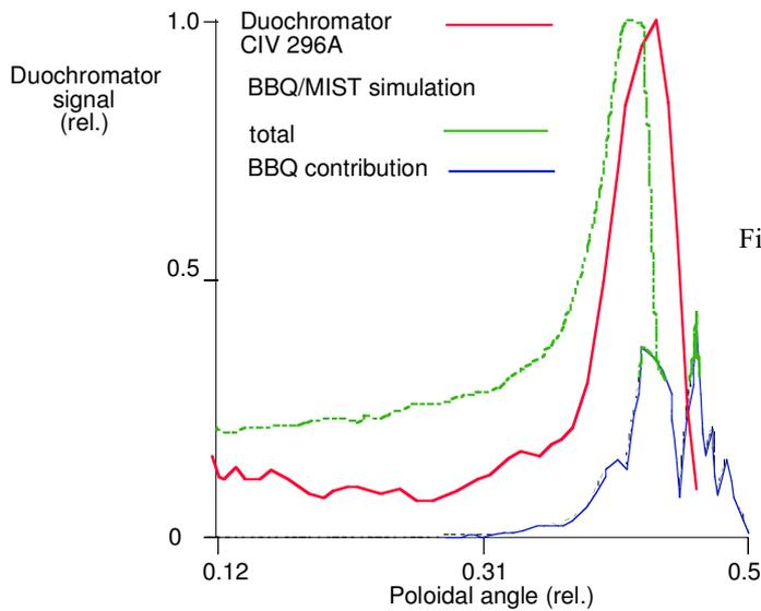
Figure 3. Comparison of measured duochromator profile for CIV with BBQ/MIST profile simulation. Data are compared with the total simulated signal and the BBQ contribution from the edge / SOL.
