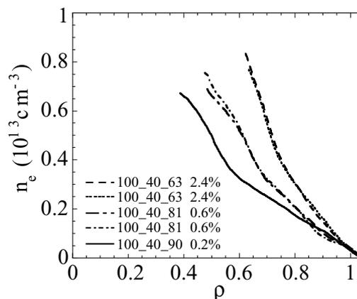
Fig. 5.- Density profiles measured in three different configurations as a function of the normalized radius.
