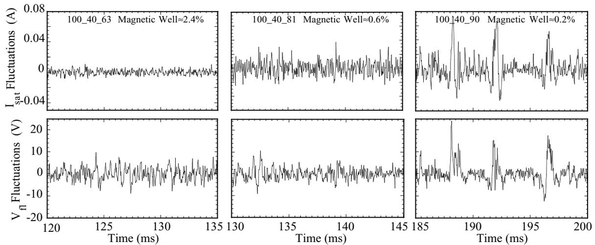
Fig. 3.- Fluctuations of the ion saturation current and of the floating potential for the studied configurations with different magnetic well in the plasma edge.
