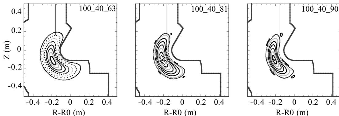
Fig. 1.- Vacuum calculations of the plasma magnetic surfaces in configurations with magnetic well 2.4, 0.6 and 0.2% respectively and similar rotational transform profile. Lines show the approximated position of the Langmuir probe.
