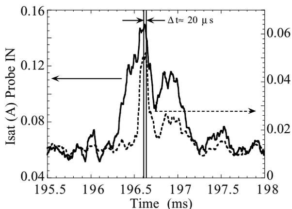
Fig. 4.- Time delay of the maximum of one of the observed events measured in two probes radially apart.
