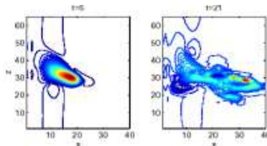
Fig. 1. The plasma density contour plots (poloidal projection) from 3D BOUT simulations.
