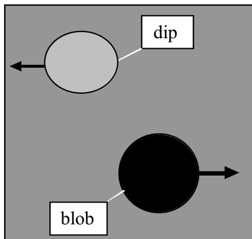
Fig. 5 Blob's and dip's convection in the SOL plasma.
