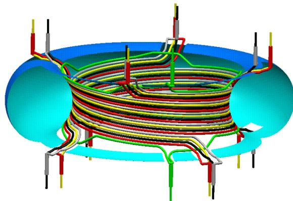
**Figure 1:** Sketch of the DED: sixteen perturbation coils located on the high field side plus two compensation coils.
