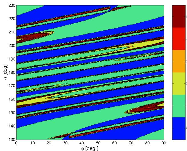
**Figure 4:** The structure of the magnetic field at the plasma wall  $r_a = 49$  cm ( $I_p = 410$  kA,  $\beta_p = 0.0$ ); close-up view of the high field side. Different colours depict different connection lengths of the field lines.
