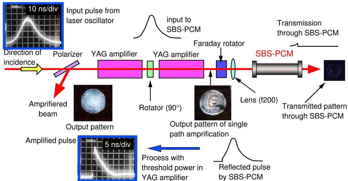
Fig.3. Schematic of double path amplification with SBS-PCM
