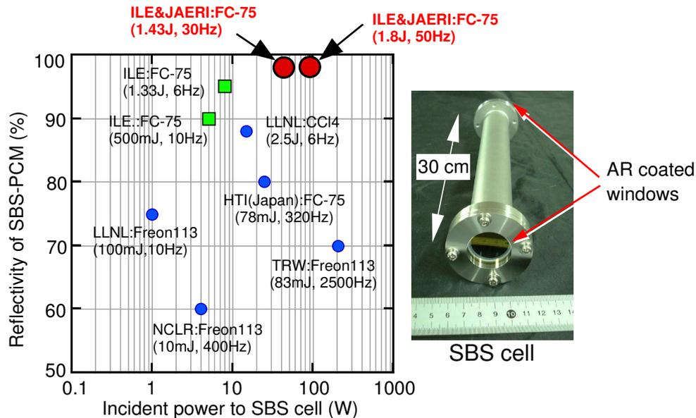
Fig.1. Reflectivity of SBS-PCM and the outside of SBS cell
