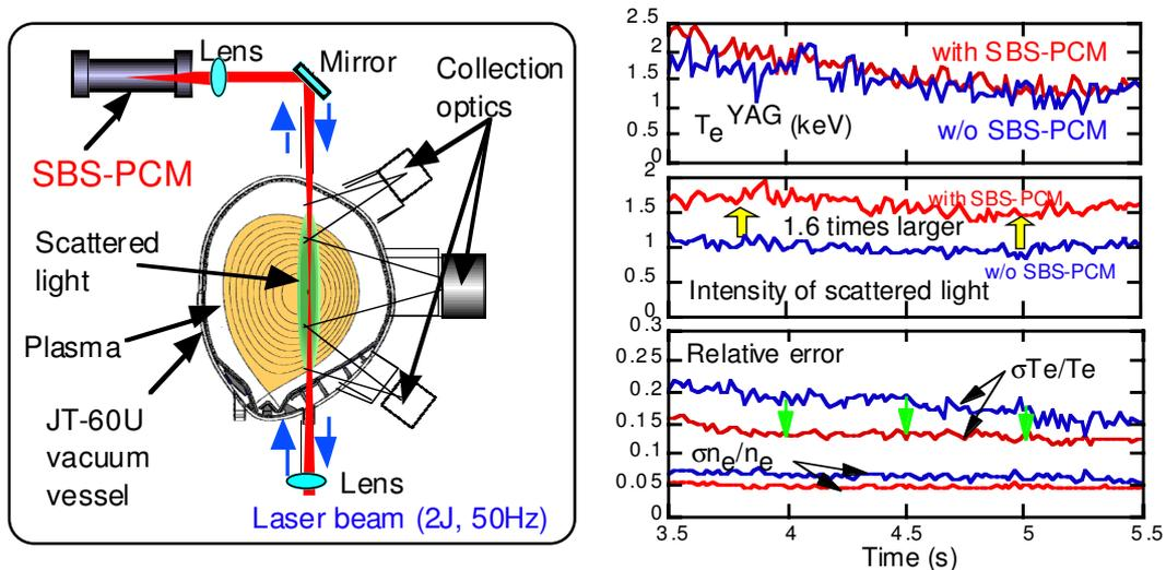
Fig.2. Schematic of double path Thomson scattering measurement and its first result
