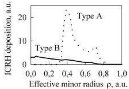
Fig. 1. The model ICRH power deposition profiles in LHD.
