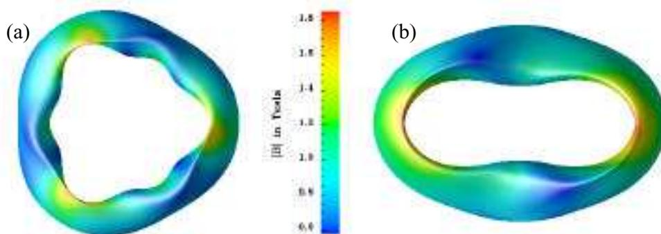
**Figure 1.** Last closed flux surface of (a) three-field period,  $\beta = 15\%$  and (b) two-field period,  $\beta = 7\%$ , quasi-poloidal symmetric stellarator configurations.
