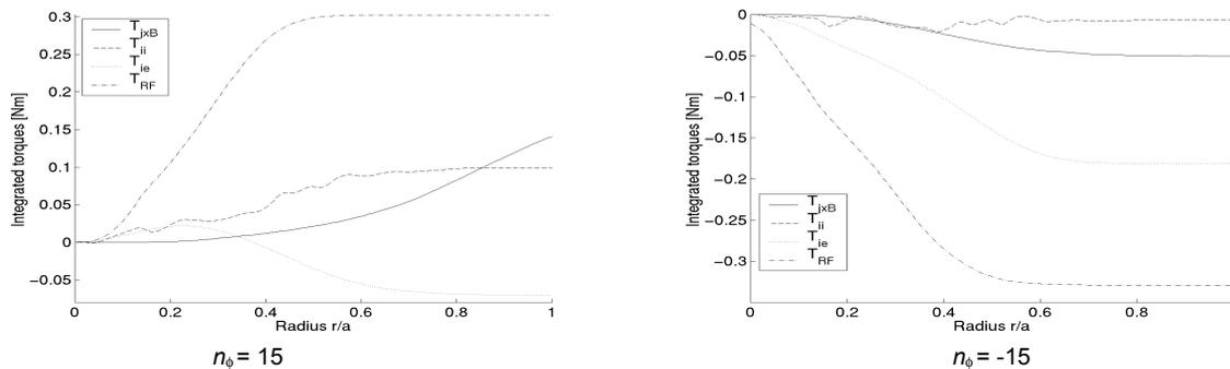
Fig. 2. The radial variation of the integrated torques  $T_{jxB}$  (full line),  $T_{ii}$  (dashed line),  $T_{ie}$  (dot line),  $T_{RF}$  (dot-dashed line) and the change in momentum of the resonant ions.
