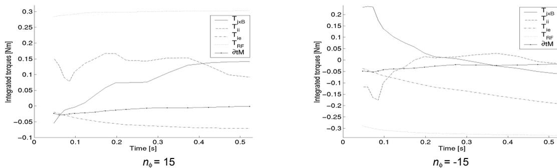
Fig. 1 Time evolutions of the integrated torques  $T_{jxB}$  (full line),  $T_{ii}$  (dashed line),  $T_{ie}$  (dot line),  $T_{RF}$  (dot-dashed line) and the change in momentum of the resonant ions (full line with points).
