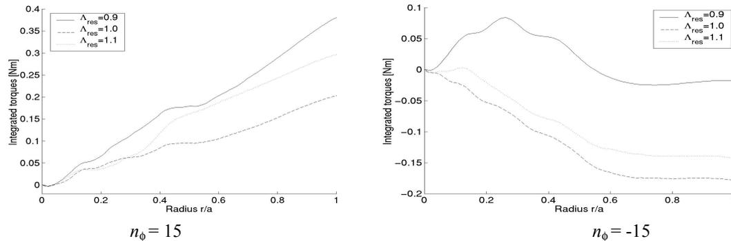
Fig. 3 The radial variation of the integrated total torques of the resonant ions for  $A_{res} = 0.9$ ,  $R_c = 2.7m$ , (full line),  $A_{res} = 1 R_c = 2.97m$  (dashed line) and  $A_{res} = 1.1$ ,  $R_c = 3.3m$ , (dotted line).
