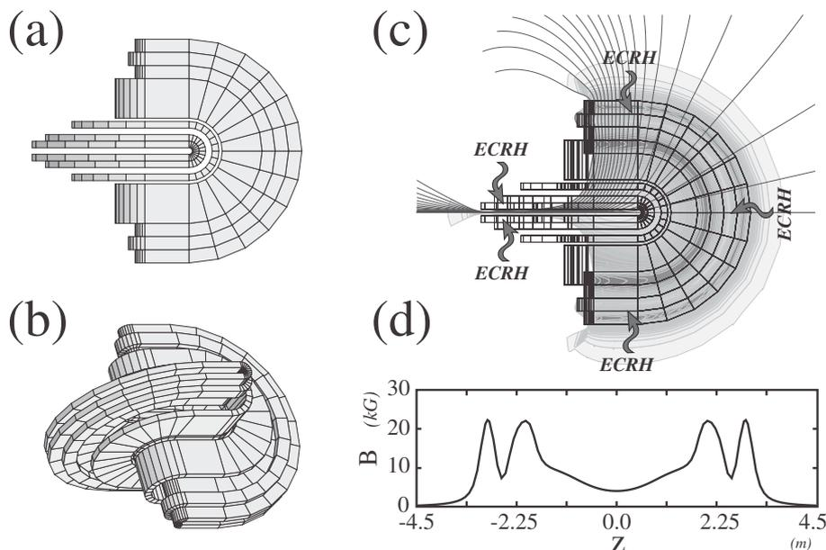
Figure 2: Schematic diagram of a single minimum-B ambipolar trap. (a) is a top view and (b) is a bird's eye view of coil system. (c) is Mod.B surfaces and magnetic field lines in a single minimum-B ambipolar trap (c) and axial profile of magnetic field (d).
