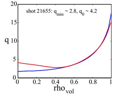
Figure 2. The reversed shear q-profile calculated by CHEASE using the current profiles of figure 1e (red curve) is compared with the “standard” profile found by the LIUQE reconstruction code (blue curve).
