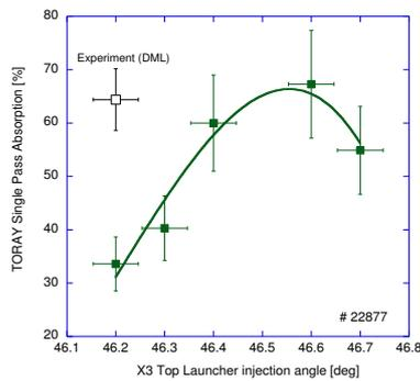
Figure 2. For this shot the X3 launch angle was fixed at  $46.2^\circ$  and the measured absorbed power was 66%. Using a launch angle of  $46.2^\circ$  TORAY-GA underestimates the absorbed power by 33%. By forcing TORAY-GA to use a launch angle of  $46.55^\circ$  agreement is obtained between the measured absorbed power and that predicted by TORAY-GA. Reasons for the discrepancy are being investigated. See main text for details.
