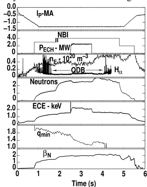
Fig. 1. Discharge conditions for QDB shot with ECH.
