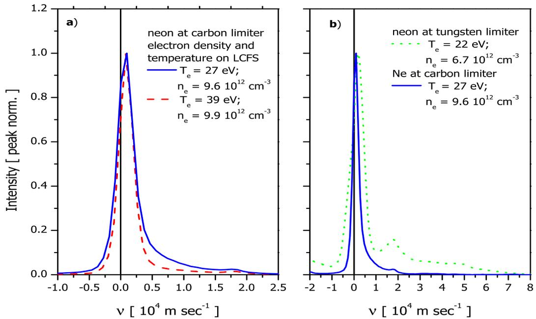
Figure 2: Velocity distribution of neon in front of a carbon and a tungsten limiter
