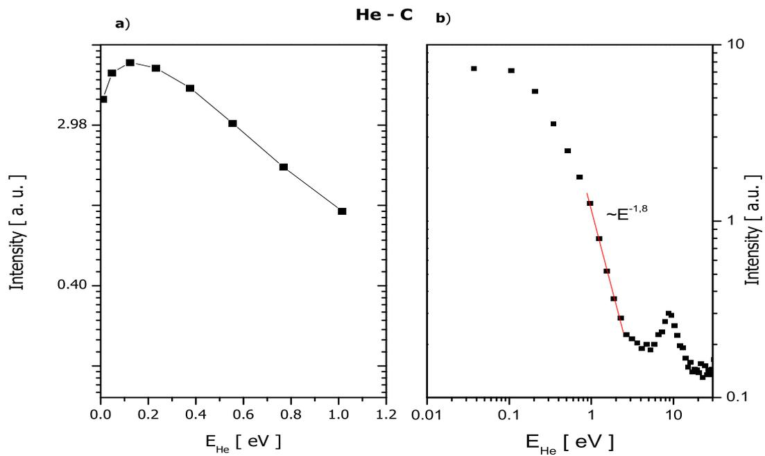
Figure 3: Energy distribution of helium in front of a carbon limiter
