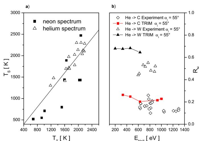
Figure 5: a) Limiter surface temperature b) particle reflection coefficient for different  $E_{HeII}$  with an ion incident angle of  $\alpha_i = 55^\circ$
