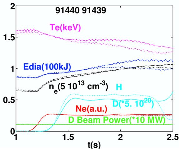
Fig 3 Evolution of the main plasma parameters in similar discharges with puff of D or H.
