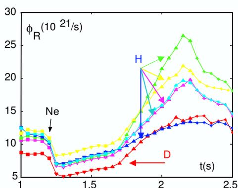
Fig 6. Time evolution of the recycling flux  $\Phi_R$  for various conditions of Ne seeding and H or D puffed from  $t=1.6$  s to  $t=2.2$  s. (idem fig 5b)
