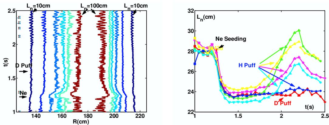
Fig 5. Evolution of characteristic lengths of the density  $L_n = |n_e / (dn_e / dr)|$
