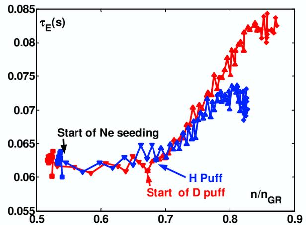
Fig. 4 Evolution of energy confinement time with  $n_e / n_{GR}$  showing difference between H and D puff.
