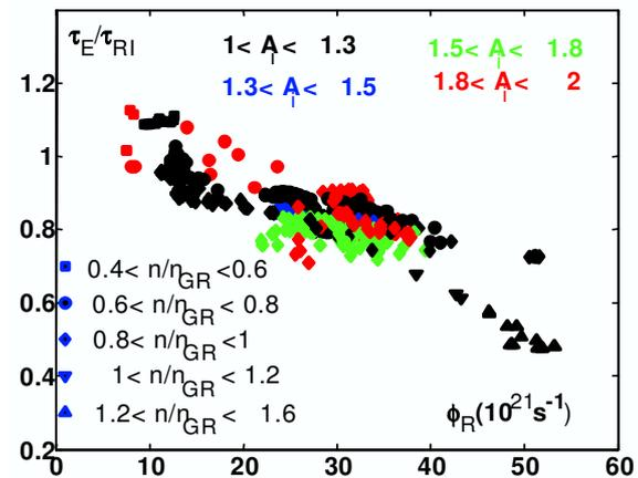
Fig. 2 Evolution of  $\tau_E / \tau_{\text{RI}}$  as function of recycling flux for different isotopic compositions of the plasma.
