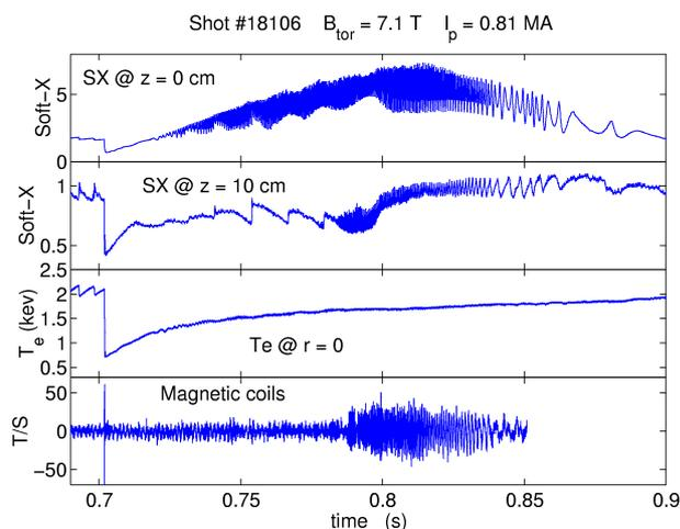
Fig. 5. X-ray traces showing that sawteeth stop and  $m=1$  mode broadens at  $t=0.78$ . Magnetic coils show the  $m=2$  mode development.
