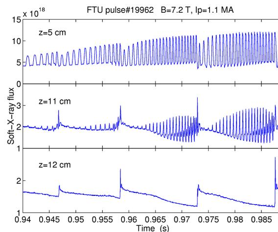
Fig. 4. Time traces showing nearly constant amplitude at  $z=5$  cm, rich harmonic content at the inversion radius ( $z=11$  cm) and no oscillations just outside ( $z=12$  cm).
