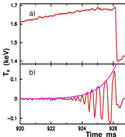
Fig. 2. Sawtooth crash with oscillating precursor (pulse #21802). a) central  $T_e$ . b)  $T_e$  oscillations near the inversion radius, and exponential with 1 ms  $e$ -folding time.
