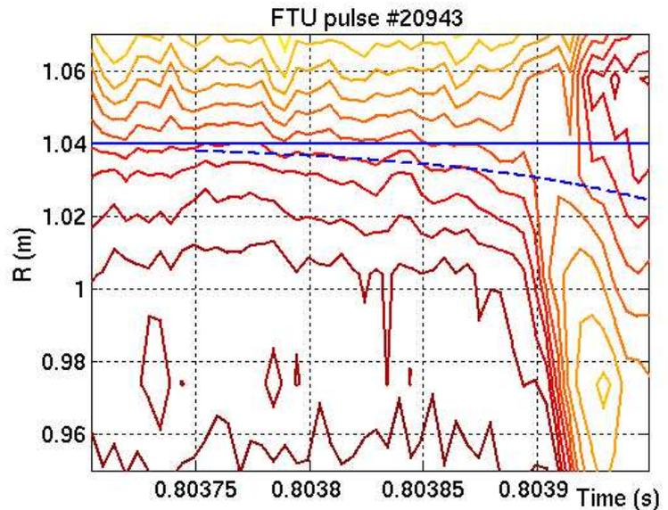
Fig. 1. Temperature contours evolution at the sawtooth crash. A growing displacement is evident before the fast collapse phase. The dashed line represents an exponentially growing displacement at the linear growth rate, the e-folding time being 97  $\mu$ s.
