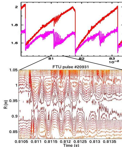
Fig. 3. Sawtooth cycles interleaved by small and large partial reconnection events. Lower frame: temperature contours showing that the displacement suddenly grows just before  $t=0.811$ .
