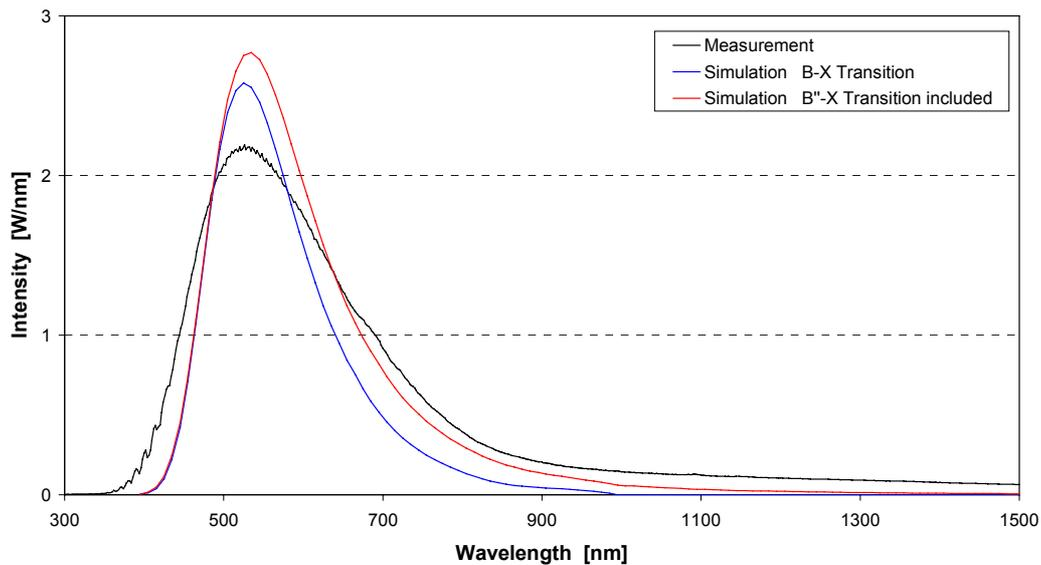
Fig. 2: Measured and calculated emission spectra.
