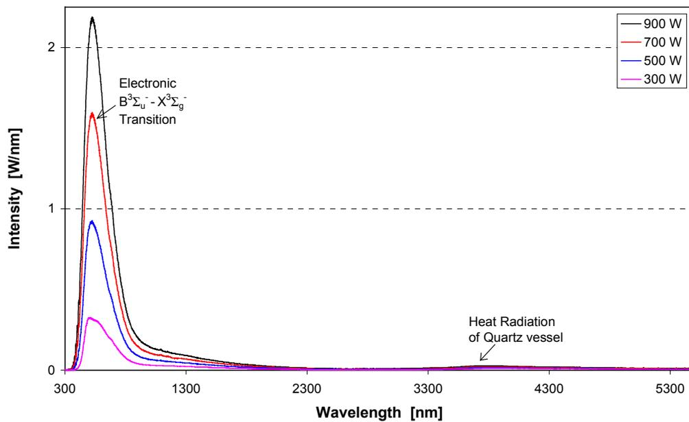
Fig. 1: Typical emission spectra of Microwave Sulfur Lamp
