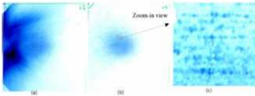
Fig.2(a)(b) are scanned RCF images showing the off-normal electron beam. (a) is the front layer and (b) is a deeper layer from the right side stack in a double-sided illumination shot. Left edge of (a) is at the target normal. (c) is a zoom of the small square in (b) showing the speckle in the beam.
