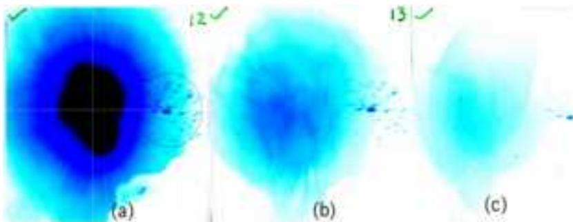
Fig.3 The raw scanned RCF images showing two separate emissions in the single sided illumination. The detector stack was about 5 cm behind the  $20 \mu\text{m}$  thick gold foil. (a) is the front layer, (b) and (c) are in the deeper layers. The off-normal beamlets are clearly visible.
