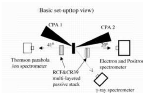
Fig.1 Schematic of the double-sided illumination experimental arrangement
