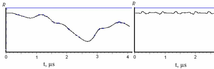
Fig. 1. Diffusion/transport process dependence upon external electric field is illustrated by ion motion in the field of the wave packet of 4 harmonics. Left figure – there is no externally applied electric field,  $K_1=1.4$ ; right case – the particle motion by the presence of electric field,  $K_2=0.6$ . Example is given for the low frequency drift waves.
