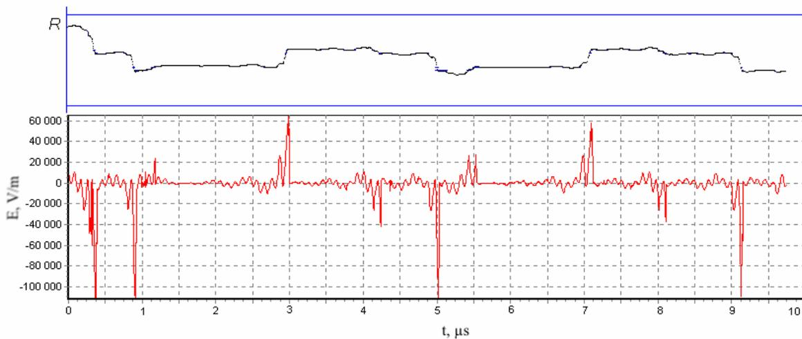
Fig. 2. Particle motion at  $K_1=1.3$ . Electric field fluctuations are in the lower hybrid drift region. For both figures the number of layers in the plasma volume is equal 5.
