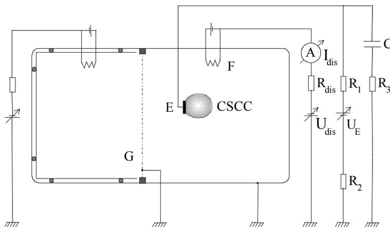
Fig. 1: Experimental set-up of the Innsbruck DP-machine.  $G$  – grid,  $F$  – filament,  $R_1 = 500 \Omega$ ,  $R_2 = 10 \Omega$ .
