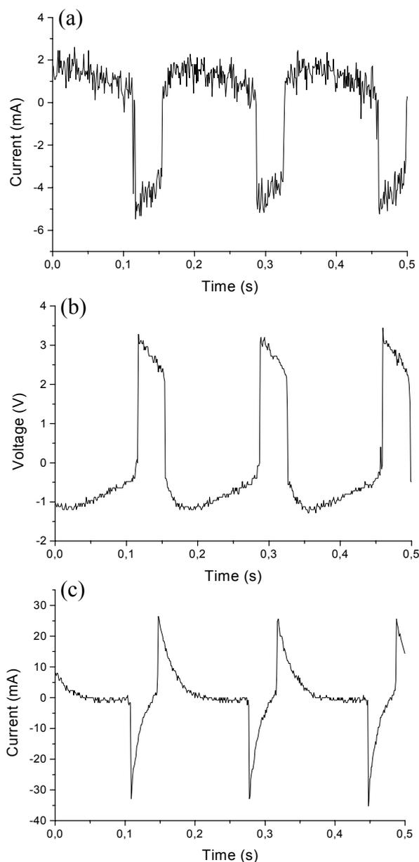
*Fig. 3: (a) Oscillation of the current in the external circuit; (b) Oscillations of the voltage across the plasma conductor; (c) Oscillations of the current in the RC branch of the circuit*
