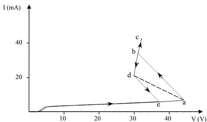
Fig. 2: Static  $I$ - $V$  characteristic obtained in DP-machine plasma.
