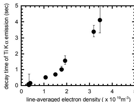
Figure 1. The dependence of the decay time of Ti K $\alpha$  emission on the line-averaged electron density in the case of balanced NBI heated LHD plasmas.
