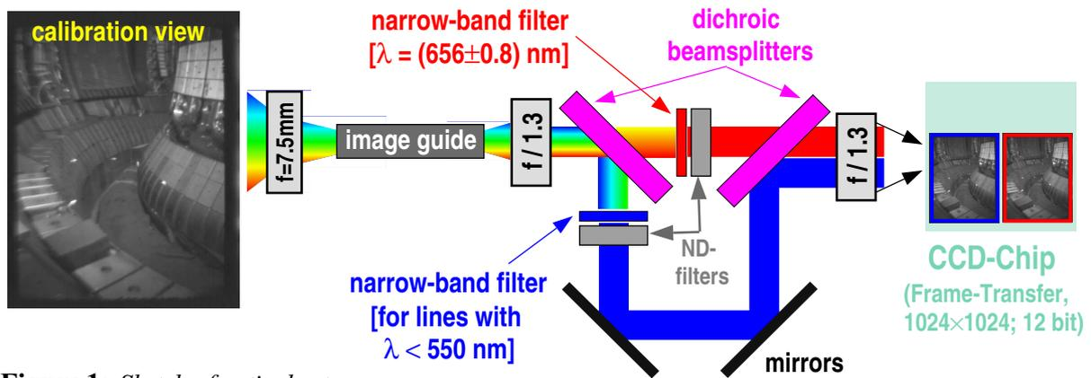
**Figure 1:** Sketch of optical setup
