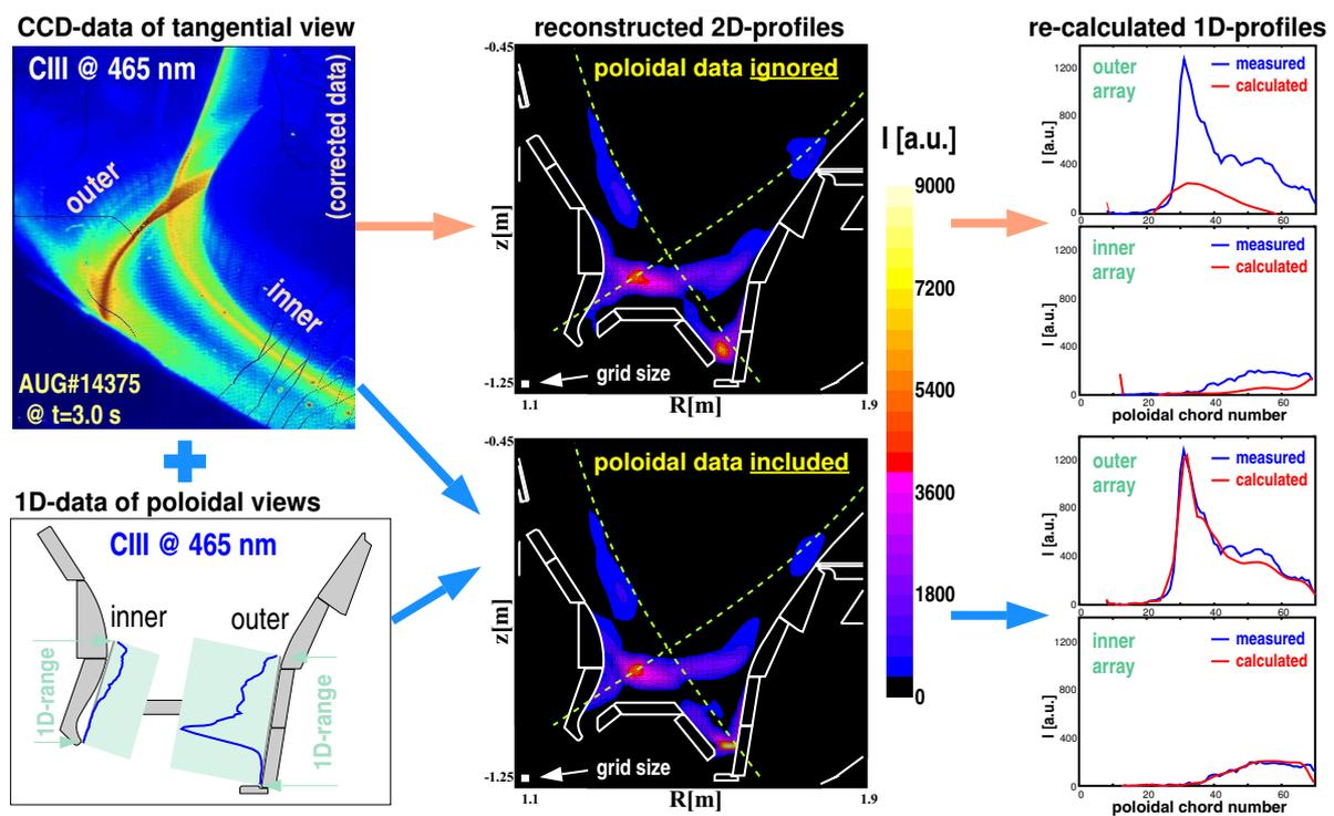
**Figure 2:** 2D-reconstruction with and without including profile information from poloidal views
