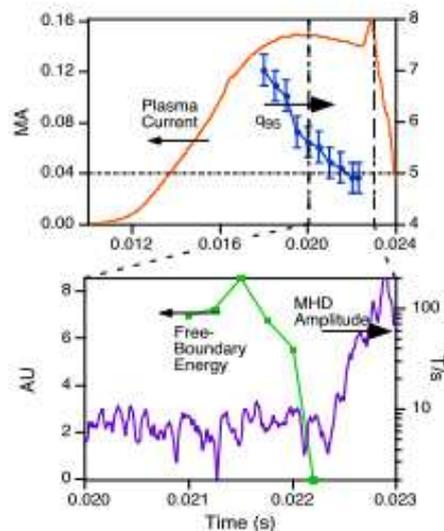
Figure 5. Characteristics of external kink mode at  $q_{95}=5$ : plasma current and  $q_{95}$  evolution through the shot, and details of mode amplitude and calculated free boundary energy prior to disruption.
