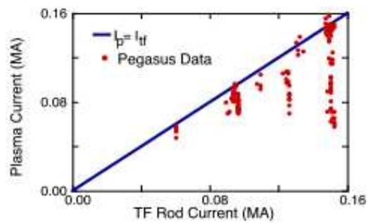
Figure 3. Plasma current vs toroidal field rod current.
