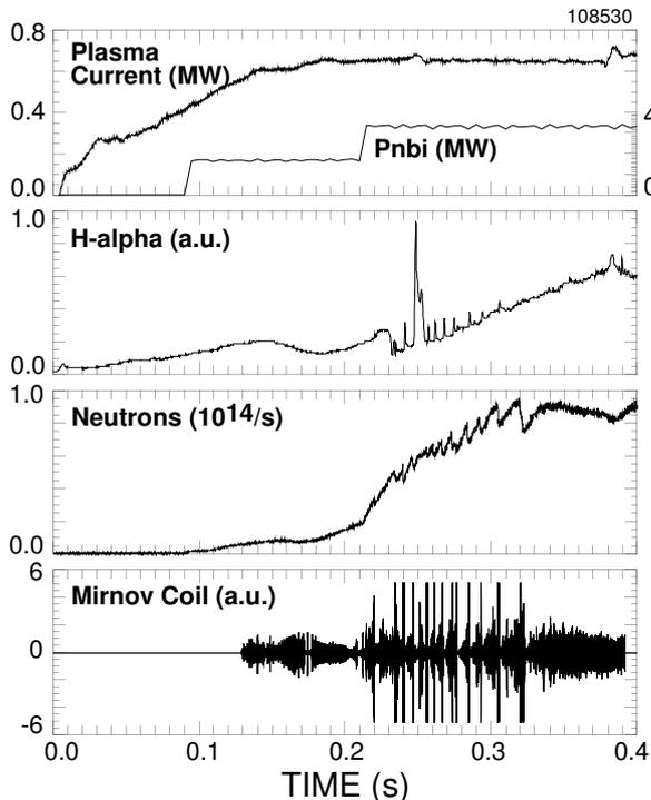
Fig. 4 Waveforms showing appearance of bursting TAE modes and fast neutron drops.
