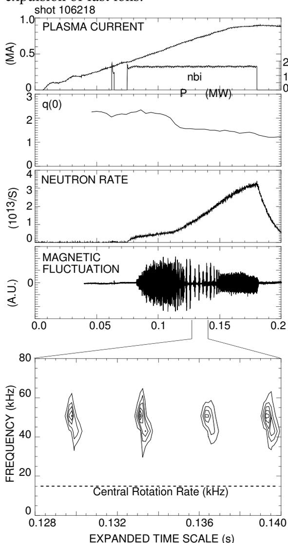
Fig. 2 Waveforms showing appearance of bounce-resonance fishbone instability.
