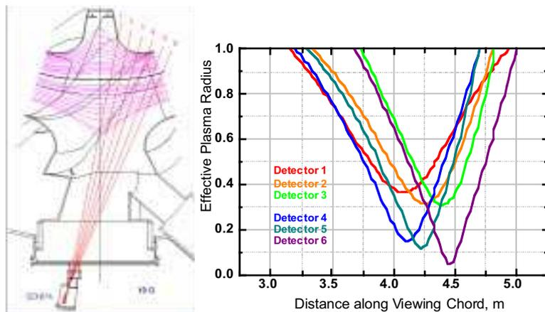
Fig. 1. Viewing geometry for the SDNPA.
