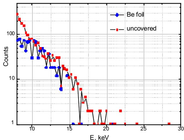
Fig. 3. Soft X-ray spectra measured by the SDNPA.
