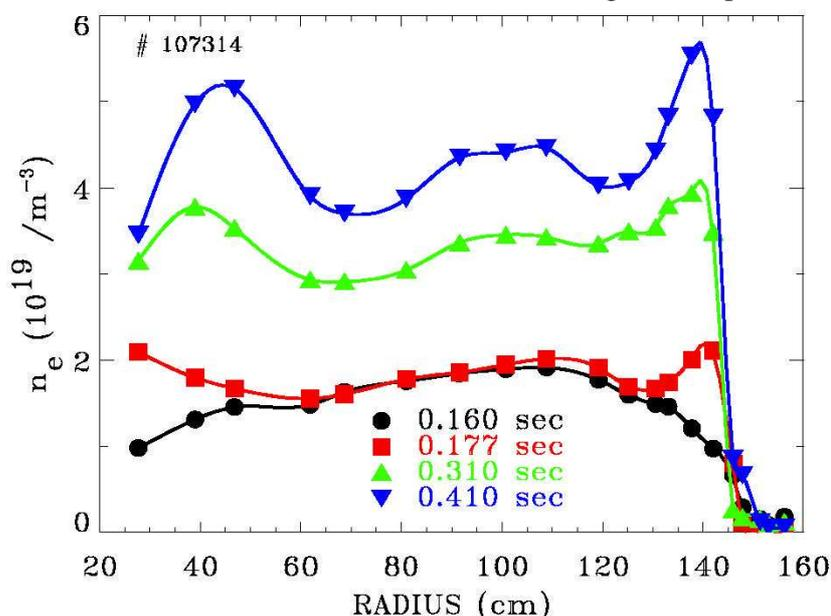
Fig. 4: Electron density profiles at several different times during a long pulse H-mode, showing development of the ears. Note  $t=0.16$ sec is in the L-mode phase.
