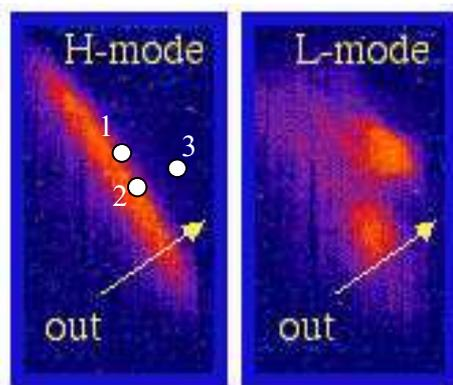
Fig.2: Images of edge turbulence in NSTX taken in HeI(587.6 nm) light with an exposure of 1 $\mu$ s. These views show a 15 cm x 30 cm region of the plasma edge in the plane perpendicular to the magnetic field, and with the outer wall toward the upper right. The plasma is relatively quiescent in the H-Mode (left), but highly turbulent in the L-Mode (right), which often shows small "blobs" which move outward in radius.
