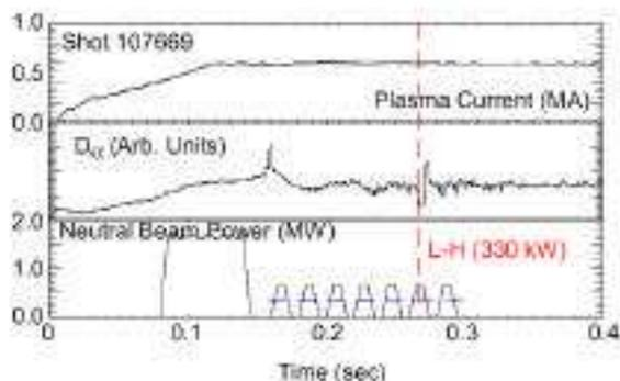
Fig. 5 Time history of NSTX discharge exhibiting the lowest power threshold to date.
