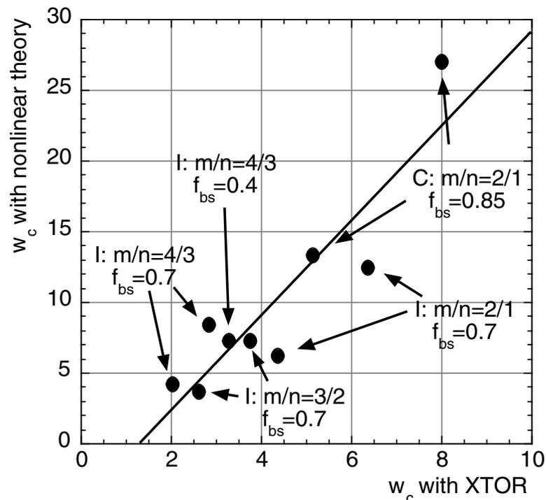
Figure 3: Nonlinear NTM marginal stability points for the circular (C) and the ITER (I) equilibria for different mode numbers,  $f_{bs}$  values and  $\chi_{\perp}/\chi_{\parallel}$  ratios.
