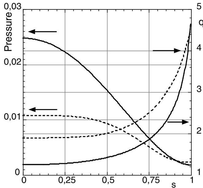
Figure 1: Equilibria pressure and safety factor profiles for **a)** the ITER (full curves) and **b)** the circular (dotted curves) case
