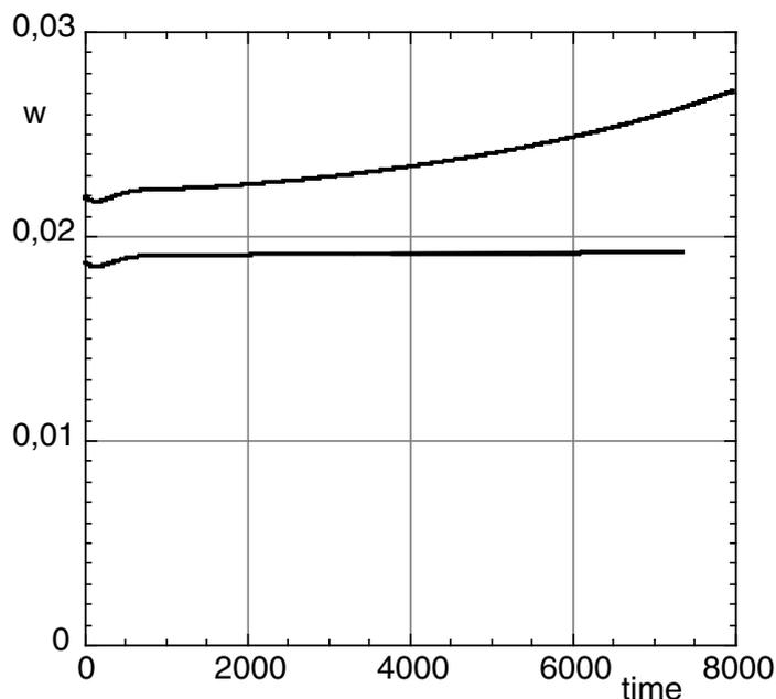
Figure 2:  $m/n = 4/3$  NTM magnetic island size time evolution for the ITER case with  $\chi_{\perp}/\chi_{//} = 10^{-8}$  with a seed island just above and below the nonlinearly unstable point.
