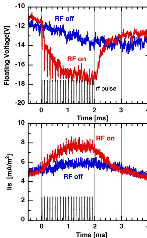
Fig. 5 Time response of  $V_f$  and ion flux of the Langmuir probe in the downstream to the heat pulse train. The rf pulse width and power are 20  $\mu$ s and 200 W, respectively.
