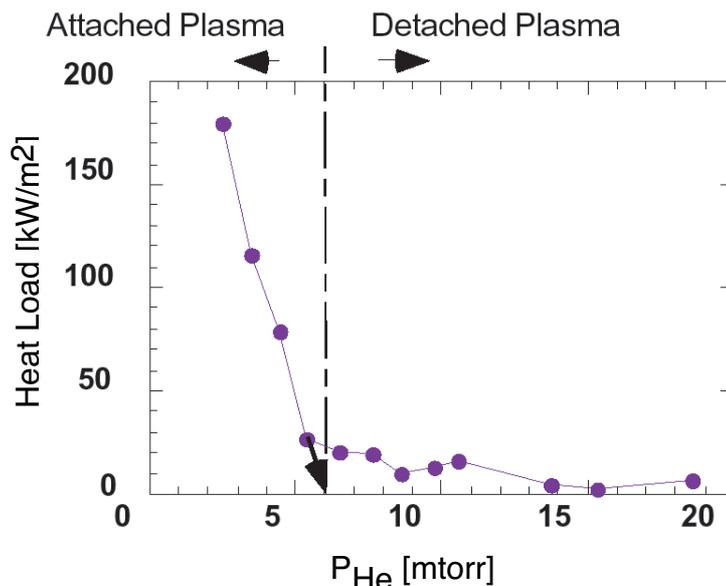
Fig. 2 Target heat flux as a function of He neutral pressure. Upstream  $n_e$  and  $T_e$  at the center are  $\sim 2 \times 10^{19} \text{ m}^{-3}$  and  $\sim 8$  eV, respectively.
