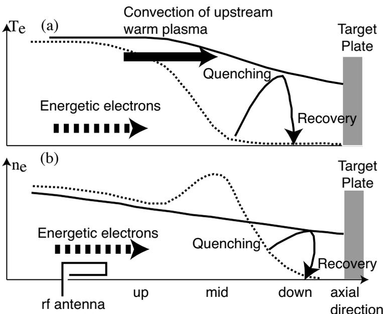
Fig. 4 Schematic structures of the dynamic behavior of the electron temperature(a) and the electron density(b) in the detached recombining plasmas accompanying with the heat pulse along the magnetic field.
