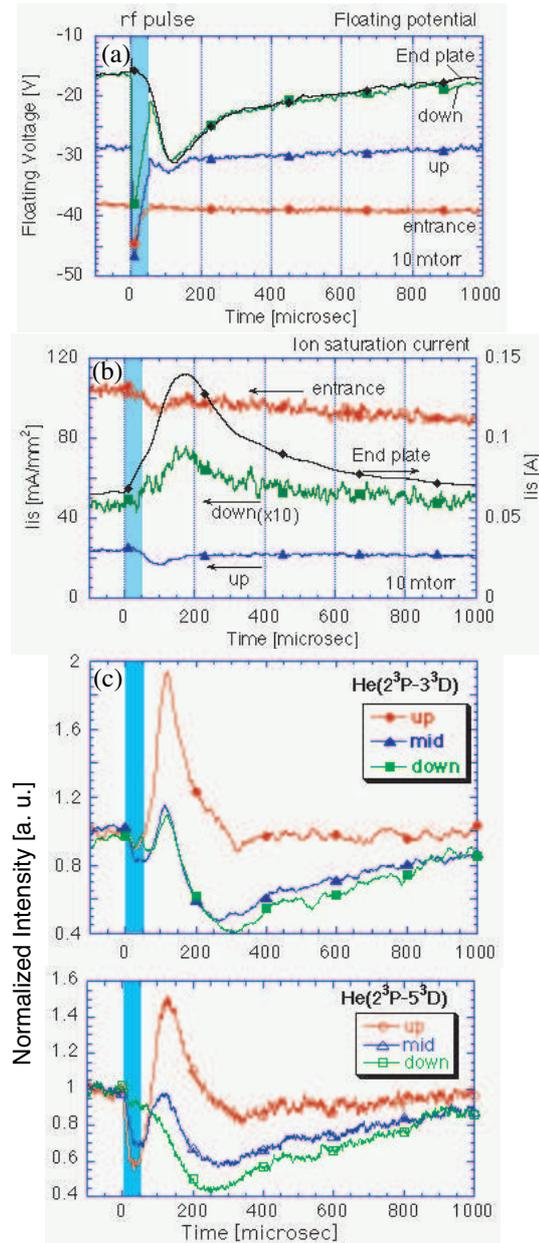
Fig. 3 Time response of the floating voltage(a), ion saturation current(b) and He Balmer series emission(c) at different axial positions. He neutral pressure is 10 mtorr and rf power and pulse duration are 500 W and 50  $\mu\text{s}$ .
