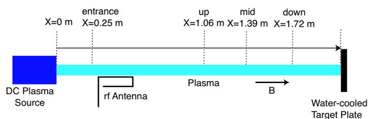
Fig. 1 Schematic configuration of the divertor simulator NAGDIS-II Axial position of probe and optical measurement and antenna position are shown.
