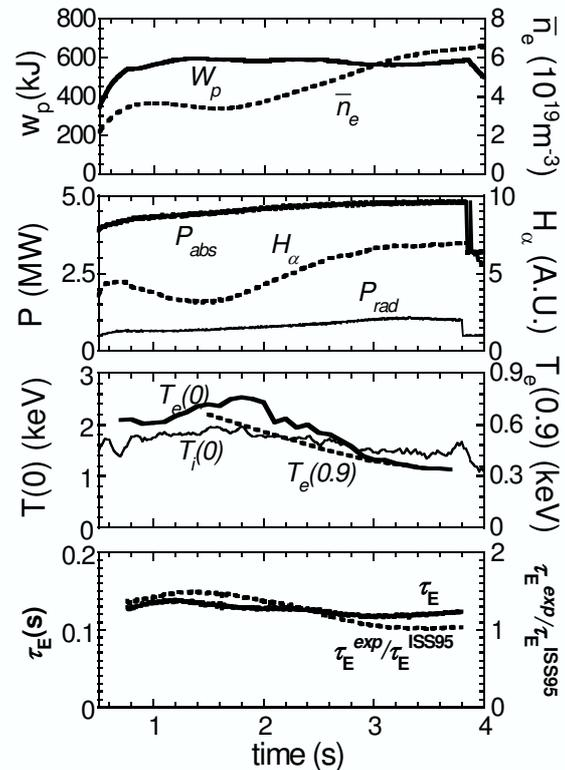
Fig.2 Waveforms of the discharge with density ramp-up. The working gas is hydrogen. Top: Stored energy and line averaged density. 2nd: Absorbed power of NBI, total radiation power, and  $H\alpha$  emission. 3rd: The electron temperatures at the center and  $\rho=0.9$  measured by the multi-channel Thomson scattering system, and the ion temperatures measured by the crystal spectrometer (Ti XXI). Bottom: Energy confinement time and improvement factor on ISS95.
