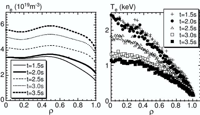
Fig.3 Left (a): Temporal change of density profile in the discharge with  $R_{ax}=3.6\text{ m}$  illustrated in Fig.2. Right (b): Temporal change of temperature profile.
