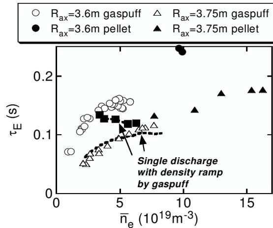
Fig.1 Dependence of energy confinement time on density in the density scan with fixed heating power. Open and Solid symbols denote gas-fueled and pellet-fueled discharges, respectively. Circles and triangles are the cases with  $R_{ax}=3.6$  m and 3.75 m, respectively. Dashed lines : time traces of single discharges with density ramp-up. The heating power is fixed at 4.5 MW and 3.6 MW in the cases with  $R_{ax}=3.6$  m and  $R_{ax}=3.75$  m, respectively.
