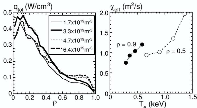
Fig.5 Left (a) : Profile of power deposition from NBI in the discharges in the case with  $R_{ax}=3.75\text{m}$ . Right (b) : Temperature dependence of thermal diffusivity at two radii of  $\rho=0.5$  (open circles) and  $\rho=0.9$  (solid circles) derived from the power balance.
