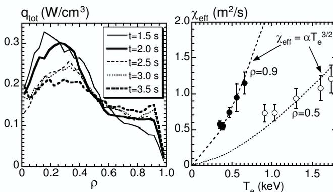
Fig.4 Left (a) : Profile of power deposition from NBI in the discharge illustrated in Fig.2 with  $R_{ax}=3.6\text{m}$ . Right (b) : Temperature dependence of thermal diffusivity at two radii of  $\rho=0.5$  (open circles) and  $\rho=0.9$  (solid circles) derived from the power balance analysis of 5 time slices.
