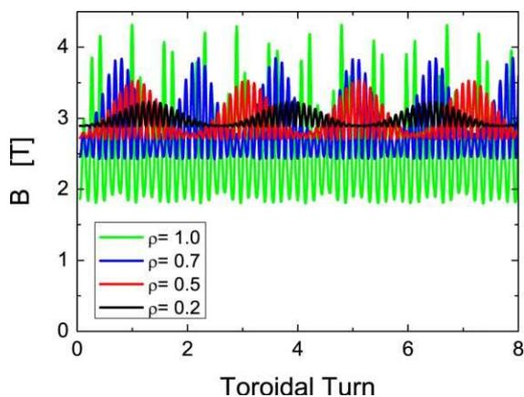
**Fig. 5** Plot of the magnetic field strength versus toroidal turn on the flux surface of  $\rho=1.0, 0.7, 0.5, 0.2$ .
