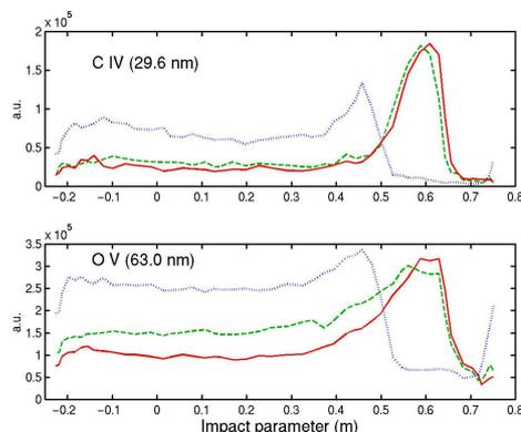
Figure 2: C IV (top) and O V (bottom) brightness profiles 0.4 s (solid line), 0.2 s (dashed) before the MARFE and after symmetrisation (dashed-dotted).
