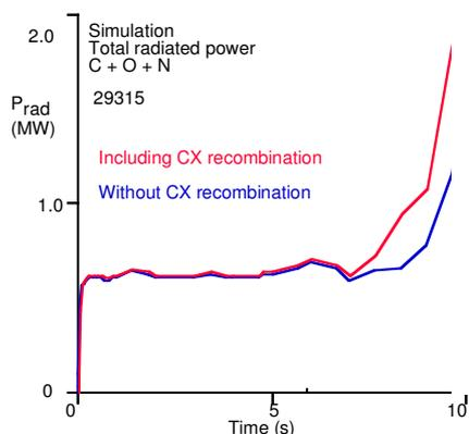
Figure 4: Simulated total radiated power with and without charge exchange
