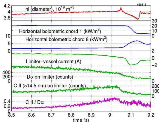
Figure 5: time traces for the identification of MARFE precursors
