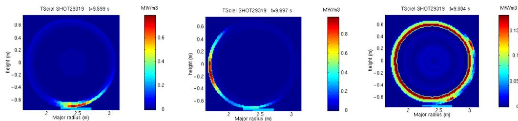
Figure 1: Tomographic reconstruction of the radiated power (left) before the MARFE, (center) during the MARFE and (right) after symmetrisation, from bolometric measurements
