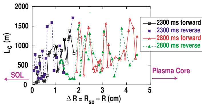
FIG. 5. Field line connection length from outboard midplane ( $\phi = 120^\circ$ ) to the vessel wall at 2300 ms (squares) and 2800 ms (triangles). Open symbols correspond to the connection length in the forward  $B_T$  direction; solid symbols correspond to the reverse  $B_T$  direction.
