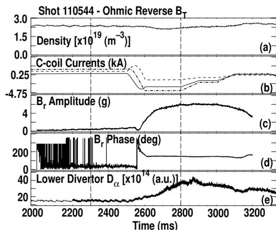
FIG. 1. Plasma response to C-coil change in discharge 110544: (a) line average density, (b) C-coil currents, radial error field (c) amplitude and (d) phase, and (e) divertor  $D_\alpha$  recycling near the outer strikepoint.
