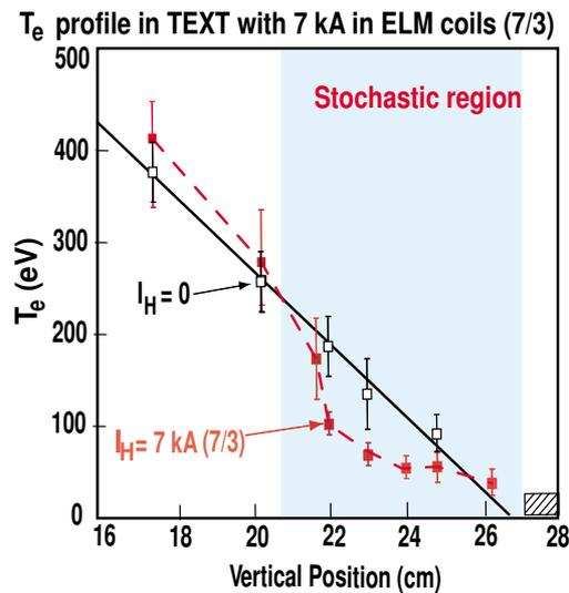
FIG. 6. H-mode-like  $T_e$  gradient formed across the stochastic layer in the TEXT tokamak with 7 kA in the Ergodic Magnetic Limiter coils [7]. The steep gradient region forms at the inner edge of the stochastic region.
