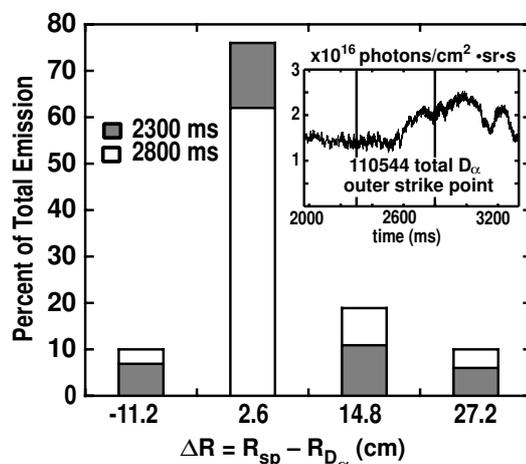
FIG. 3. Broadening of the  $D_\alpha$  profile when the stochastic layer is formed. Inset shows the increase in overall recycling.  $\Delta R$  is the distance of the  $D_a$  measuring chord from the strikepoint.
