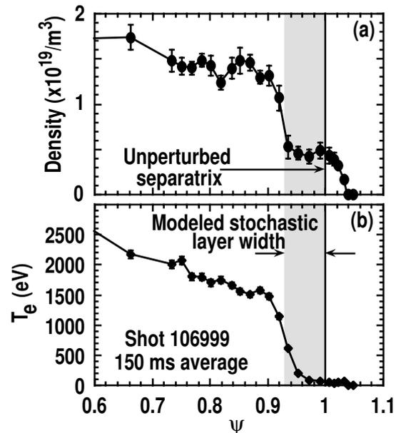
FIG. 7. Plasma density (a) and  $T_e$  (b) profiles from Thomson scattering for QDB shot 106999 showing flat regions at the edge coincident with the stochastic layer width modelled with TRIP3D.
