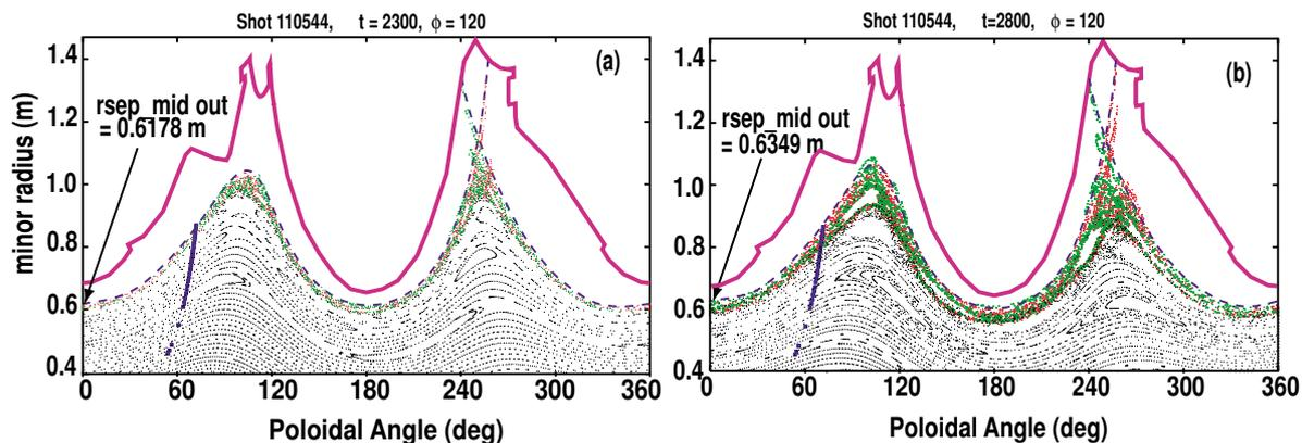
FIG. 4. TRIP3D results for DIII-D discharge 110544 at (a) 2300 ms and (b) 2800 ms. Black dots represent field lines that do not cross the unperturbed separatrix. Red and green dots represent field lines integrated in the forward (red) and reverse (green)  $B_T$  direction that intersect a material surface.
