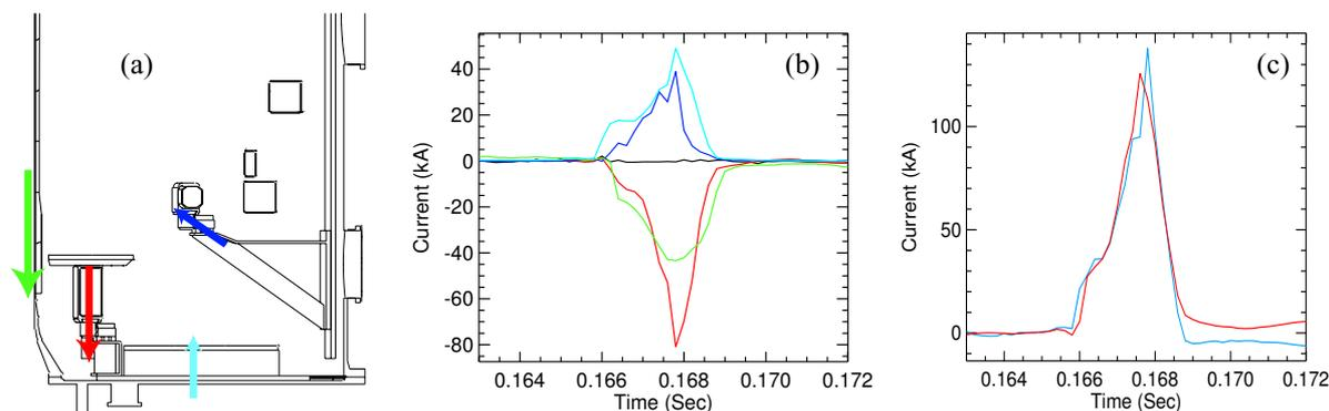
Figure 2: Halo current evolution for shot 3819, a downward VDE with plasma current just prior to the VDE of  $\sim 600$  kA.
