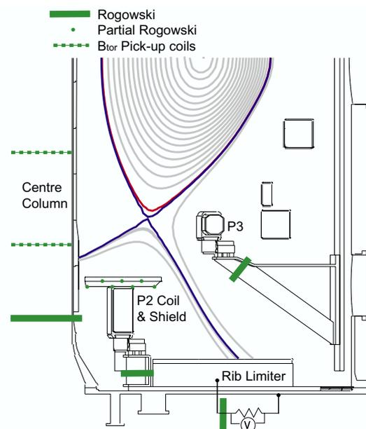
Figure.1 Schematic of divertor region of MAST vessel showing position of halo current detectors.
