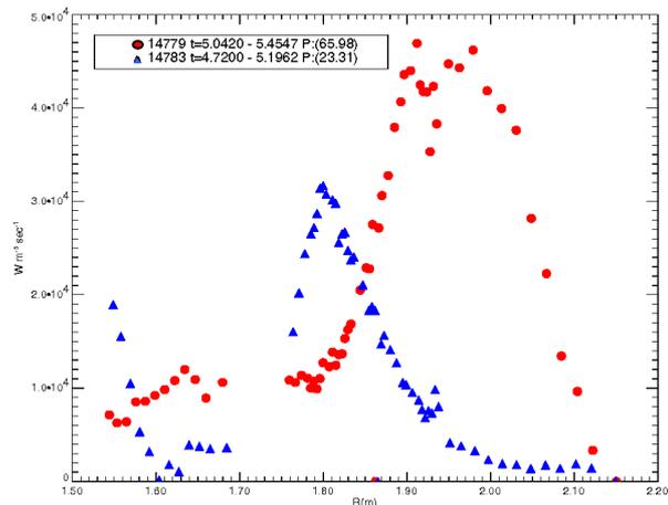
Fig. 4: direct damping on electrons deduced from ICRF power modulation for shots # 14779 (red circles) between 5 and 5.5 s and # 14783 (blue triangles) between 4.7 and 5.2s
