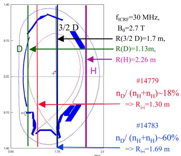
Fig. 1: positions of the different ion cyclotron resonance layers
