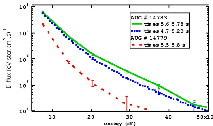
Fig. 5: D fluxes measured by Neutral Particle Analysers at different times intervals for shots #14779 (red dashed line) and #14783 (green line and blue dots)
