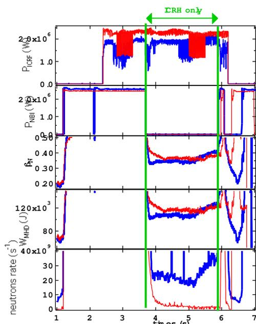
Fig. 2: times traces of shots # 14779 (red) and # 14783 (blue); a/ ICRH power, b/ NBI power, c/ poloidal beta, d/ MHD energy content, e/ neutron flux
