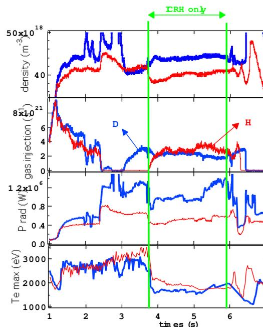
Fig. 3: times traces of shots # 14779 (red) and # 14783 (blue); a/ line averaged density, b/ gas injection (H for #14779, and D for #14783), c/ radiated power, d/ maximum electron temperature from ECE Michelson interferometer
