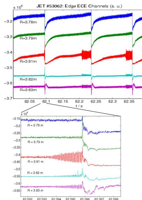
Figure 4: Edge ECE signals showing the coherent precursors.
