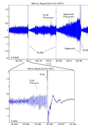
Figure 1: Mirnov signals of a low field side coil.
