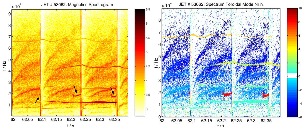
Figure 2: Magnetics spectrogram of a coil located on the low field side with the precursors being marked by the arrows, and spectrum of toroidal mode numbers showing the modes to have  $n=8$  (red).
