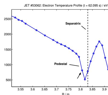
Figure 5: Electron temperature profile as measured by the ECE.
