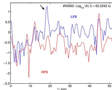
Figure 3: Logarithmic Fourier spectra of Mirnov signals of low/high field side coils with comparable distance to the separatrix. The arrow points at the precursor contribution.
