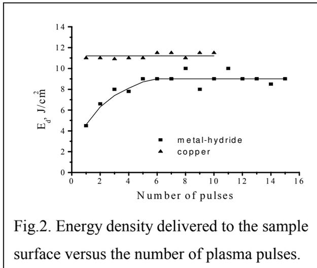
Fig.2. Energy density delivered to the sample surface versus the number of plasma pulses.
