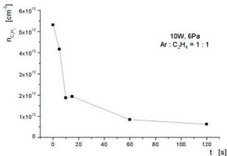
Fig.3: Decrease of the C<sub>2</sub>H<sub>2</sub> absorption by decomposition of the precursor gas.
