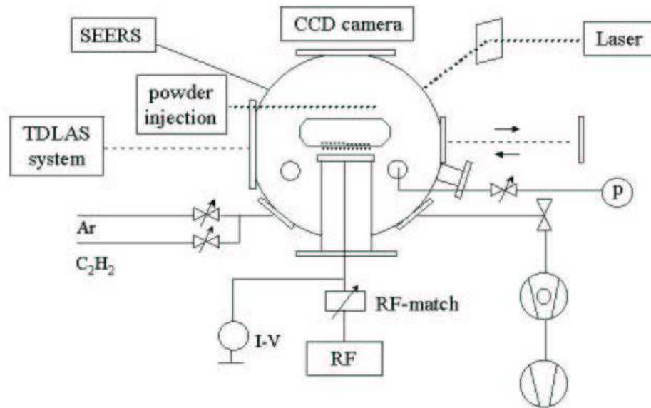
Fig.1: Scheme of the experimental set-up PULVA1.
