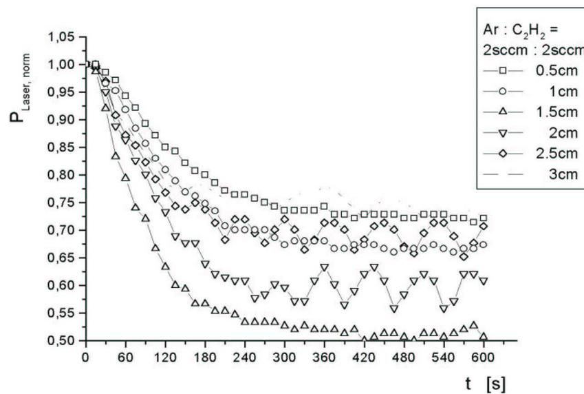
Fig.4: Decrease and oscillation of the laser light due to the growth and the dynamics of the particles at different heights above the rf-electrode.
