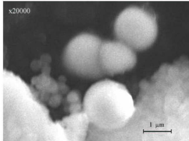
Fig.2: a-C:H coated SiO<sub>2</sub> particles (middle) and synthesized small carbon particles which form large clusters (left and right).
