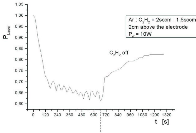
Fig.5: Vanishing particle density after stop of  $C_2H_2$  supply.
