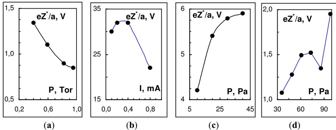
**FIGURE 4.** The effective dust charges  $Z^*$  for different experiments in dc- (a),(b) and rf - (c), (d) discharges under (a),(c) ground-based and (b),(d) microgravity conditions.
