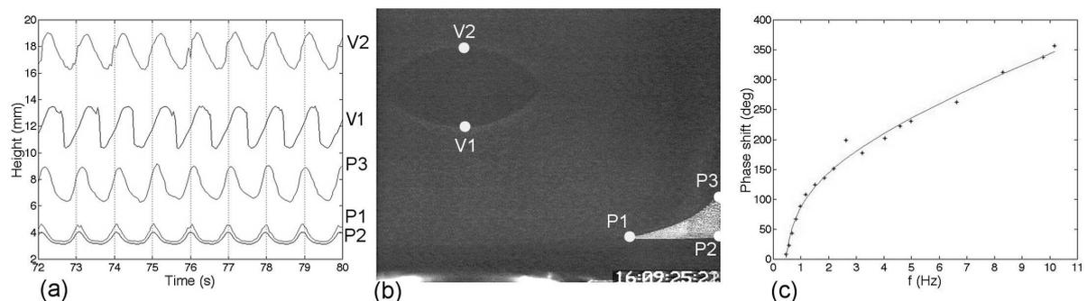
**FIGURE 3.** Low frequency excitation of a cloud constituted of grown and  $3.4\ \mu\text{m}$  particles, a) time evolution of the height of the points labeled in b), c) measurements of the phase shift between V1 and P1
