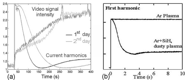
**FIGURE 2.** Time evolution of the current harmonics, a) on board with video signals, b) in an Ar-SiH<sub>4</sub> plasma
