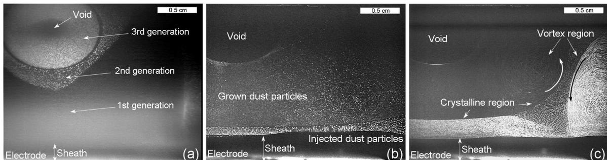
**FIGURE 1.** Dust clouds on ground : a) multiple generations, b) grown and injected particles ( $3.4 \mu\text{m}$ ), c) crystalline and vortex-like regions of various sizes grown particles (15 images superimposed)
