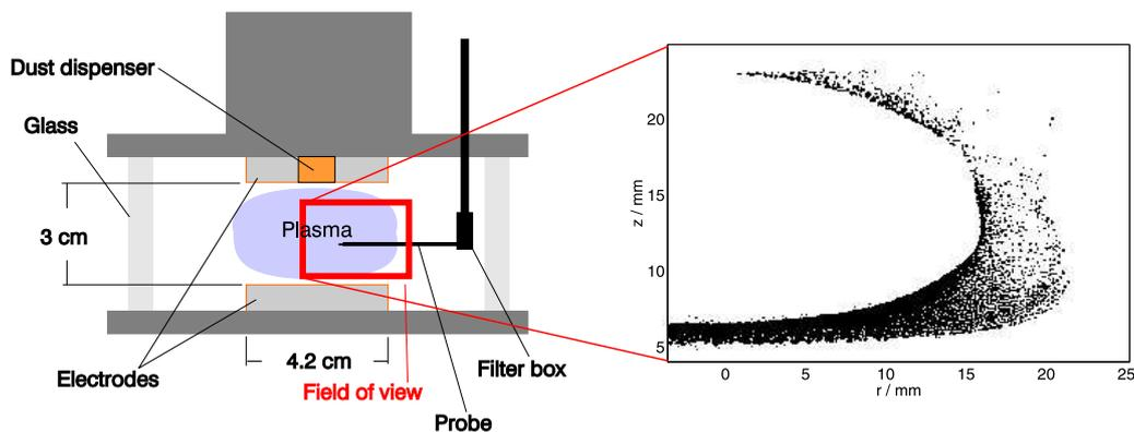
Figure 1: Scheme of the discharge chamber, camera field of view and dust distribution for the parameters of the presented experiment.
