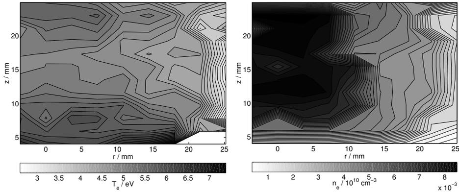
Figure 3: (a) electron temperature and (b) electron density for  $p = 37.5 \text{ Pa}$  and  $U_{rf} = 80 V_{pp}$ .
