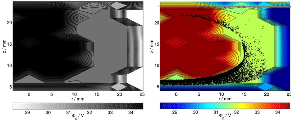
Figure 2: (a) plasma potential and (b) the plasma potential profile with the superposed particle cloud. The electrodes extend to  $r = 21$  mm.
