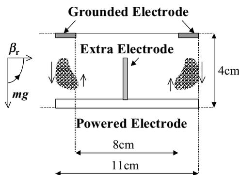
Figure.1 Experimental set up for vertical vortex producing
