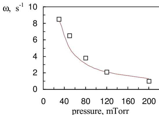
Figure 2. The dependency of rotation frequency  $\omega$  on the pressure. The points are the experimental values, solid line corresponds to  $\omega = g/4P$  [mTorr].
