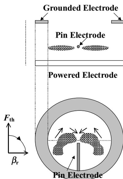
Figure 3. Simplified schematic diagram of the apparatus used for the formation of horizontal dust vortex
