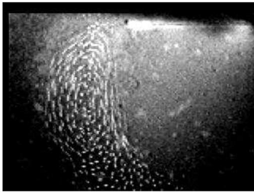
Figure 4. Typical video image of dust vortex
