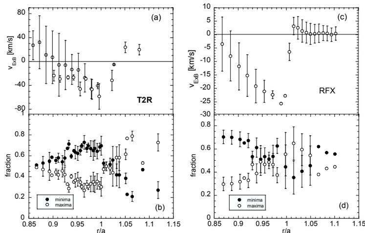
**Fig 2** Average  $v_{ExB}$  radial profile (a), relative fraction of minima/maxima (black/open symbols) events vs radial position (b), data from T2R; analogous data respectively in (c) and (d) from RFX
