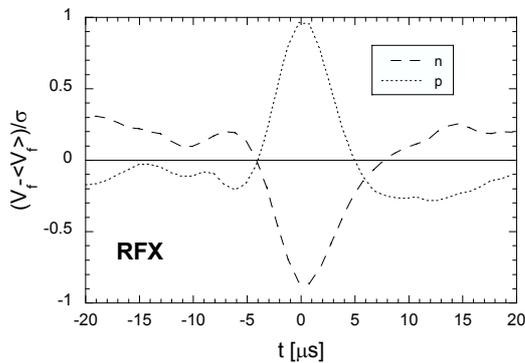
**Fig 1** Conditional average based on events located at 10  $\mu\text{s}$  time scale on  $V_f$  signals; data from RFX
