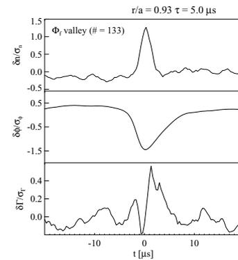
**Fig 3** Conditional average on electron density, floating potential and electrostatic particle flux based on events located at 5  $\mu\text{s}$  time scale on  $V_f$  signals; data from T2R
