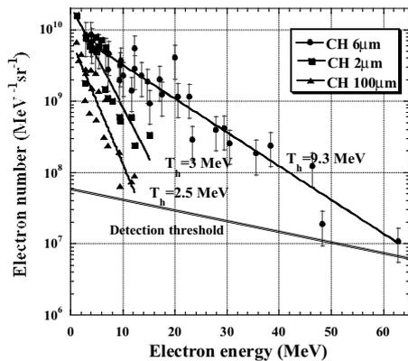
Fig. 1: Experimental electron energy distributions measured at  $0^\circ$ .
