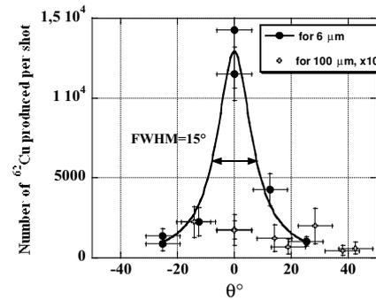
Fig. 2 : Number of  $^{63}\text{Cu}(\gamma,n)^{62}\text{Cu}$  reactions produced per shot using 6 and 100  $\mu\text{m}$  thick CH target .
