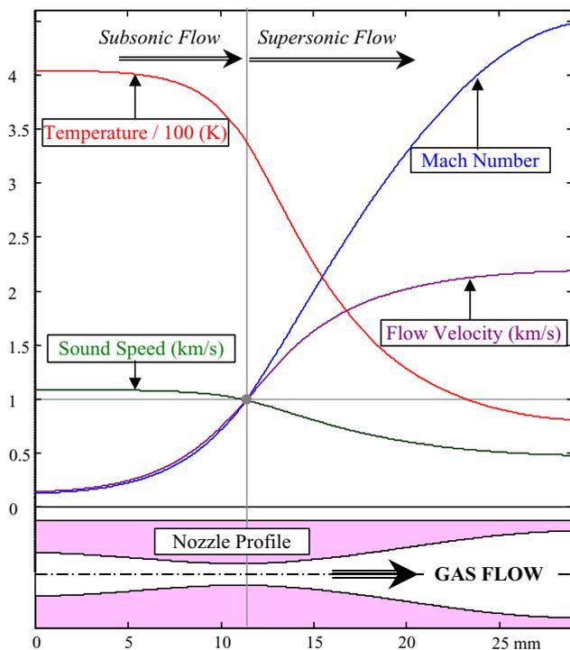
Fig. 1. Gas flow through a Laval nozzle in supersonic regime.
