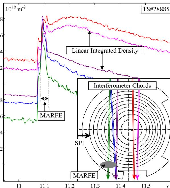
Fig. 3. Evolution of interferometer chords during SPI
