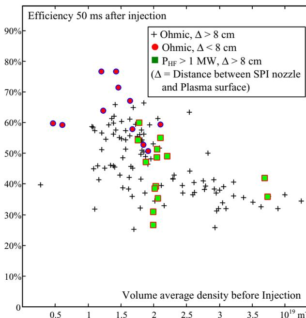
Fig. 4. Fuelling efficiency of SPI, as a function of the density.
