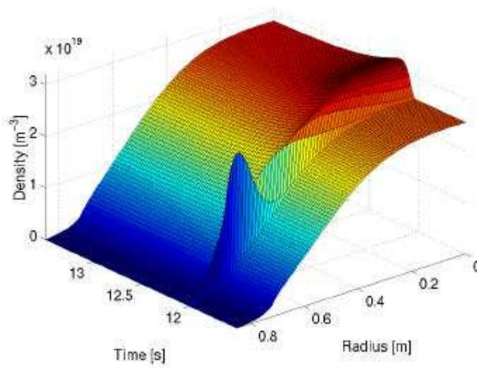
Fig. 7. Density profile evolution during SPI injection
