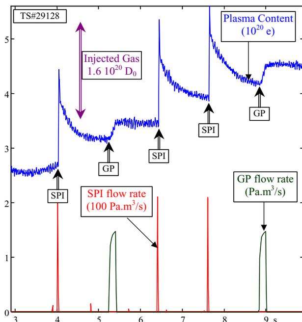
Fig. 2. Pulsed gas injection with GP and SPI
