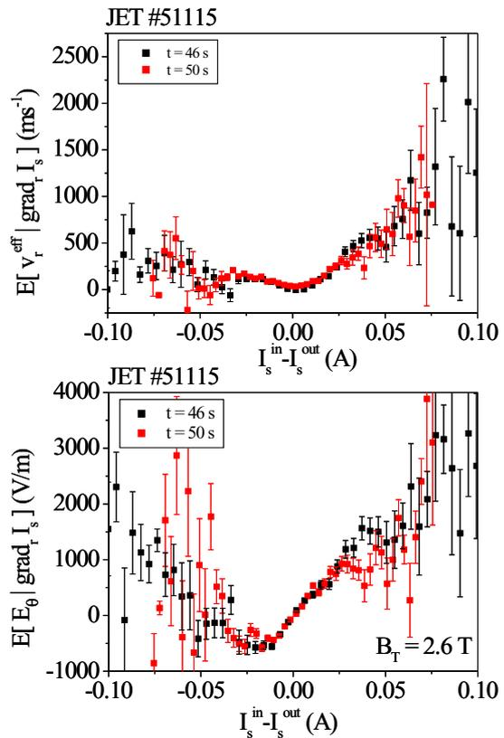
Fig. 4: (a) Effective radial velocity versus fluctuations in the radial gradient; (b) Poloidal electric fields versus radial gradient. Measurements were taken at  $r - r_{LCFS} \approx 1$  cm.
